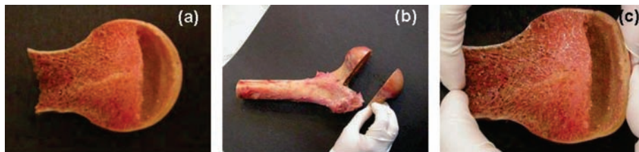
FIGURE 11.11. A, partially cored out femur mimics a postoperative avascular necrosis of the femur. B, the “halves” of the femoral neck and head are fitted back together after the creation of the cavity. C, the cavity permits deformation, with compression, of the femoral head.
