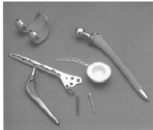
Figure 3. Different materials made from stainless steel. Used in orthopedic implants [8].
